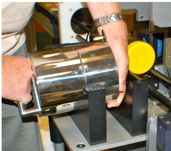
**To load the source on the MSCL in a vertical orientation**
